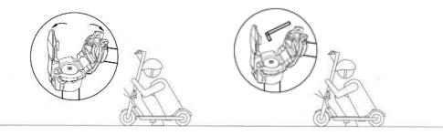
If your standpipe in electric scooter is shaking, please use the M5 hex wrench to lock the two screws at the fold mechanism.
