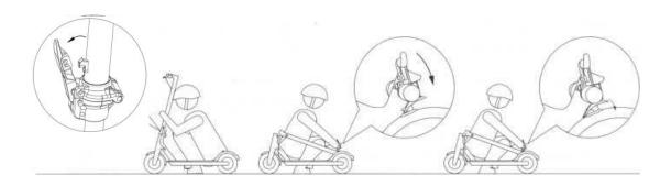
Make sure that the electric scooter is turned off, standpipe will dip through folding, open the folding wrench, and aim at the bell position and hook the bell with the rear mudguard. When opening you need to press the bell hook at the hook, until the bell hook is out of the stall after the hook, the vertical standpipe and lock folding plate back to fold.
